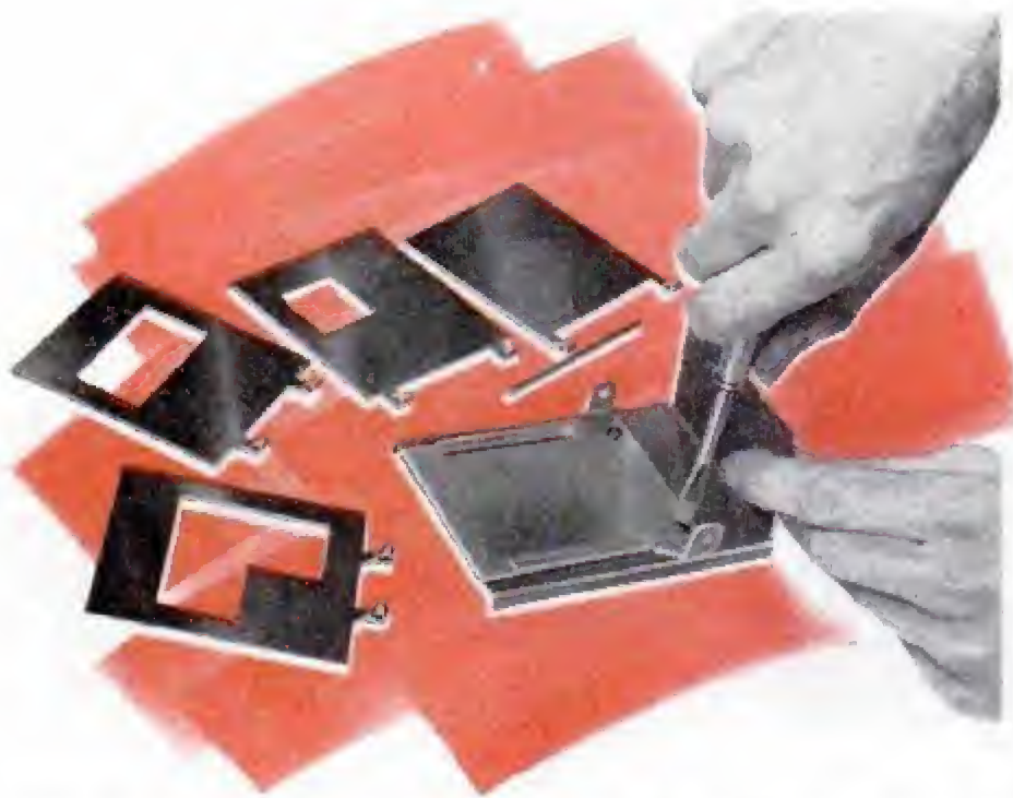
Here are all the parts cut and ready for final assembly. Two sheet-metal screws are used to fasten the paper holder to the base member
